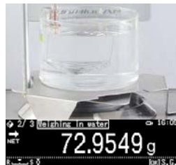
Then place it in the container filled with water, as instructed on the screen.
