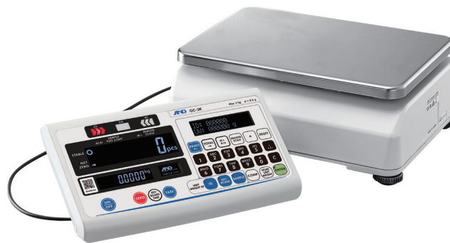
Display unit detached from the weighing unit
